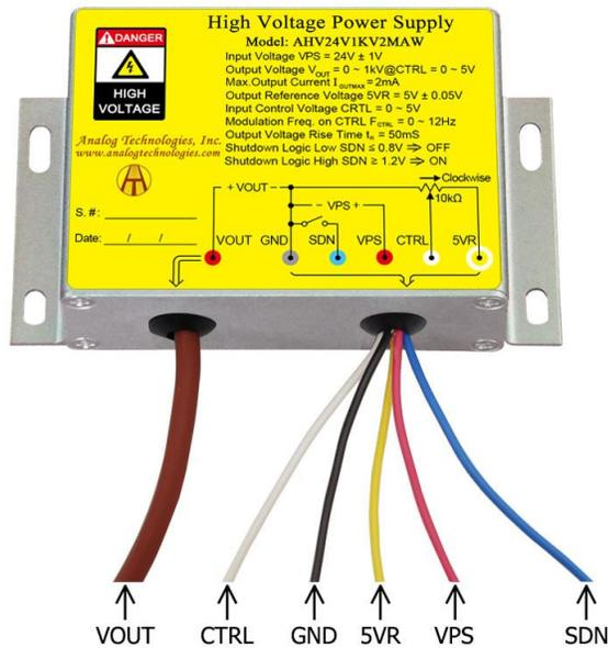
Figure 2. The Connecting Lead Wires of AHV24V1KV2MAW
