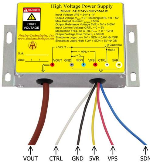
Figure 2. The Connecting Lead Wires of AHV24V2500V5MAW
