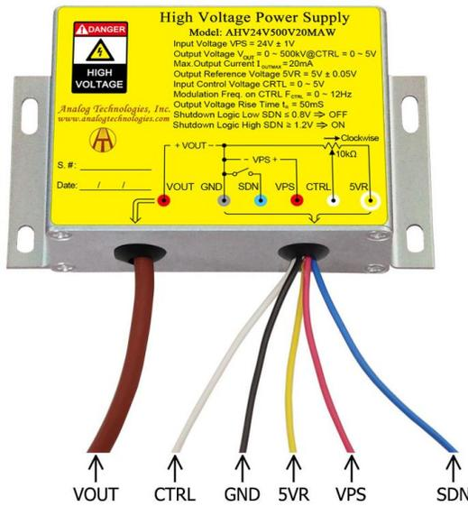
Figure 2. The Connecting Lead Wires of AHV24V500V20MAW
