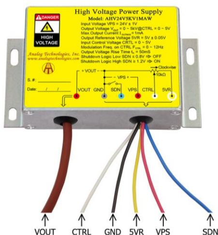
Figure 2. The Connecting Lead Wires of AHV24V5KV1MAW
