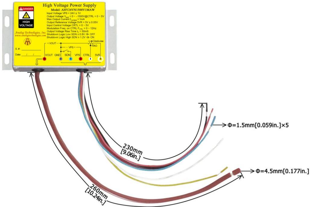
Figure 13. Connecting Lead Wires of AHV24VN1500V1MAW
