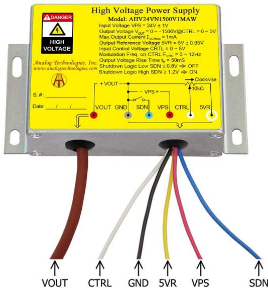
Figure 2. The Connecting Lead Wires of AHV24VN1500V1MAW
