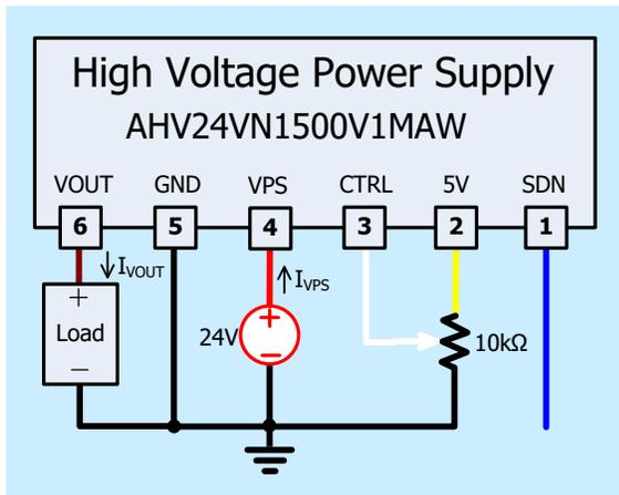
Figure 3. Setting Output to be a Constant Voltage
