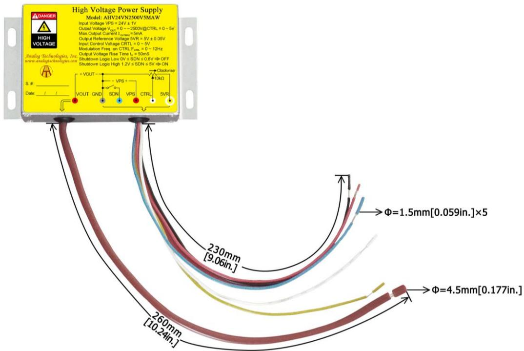
Figure 13. Connecting Lead Wires of AHV24VN2500V5MAW
