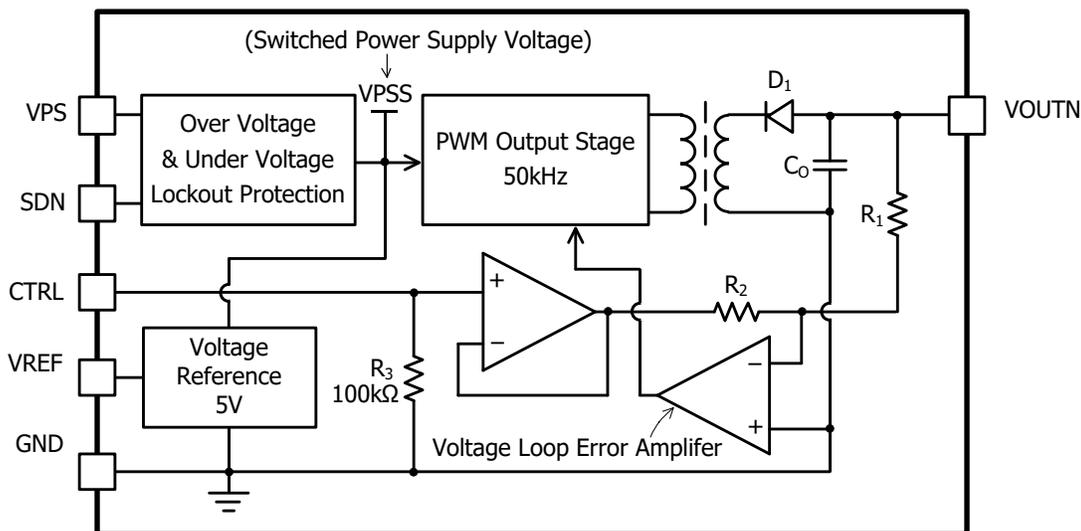
$V_{OUTN} = -N \times V_{CTRL}$ , where N is the amplification factor:  $N = R_1/R_2$ .
