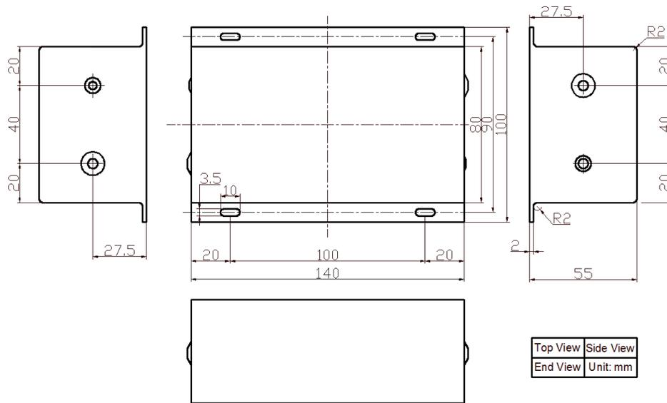
Figure 11. Dimensions for AHV24VN25KV1MAW
