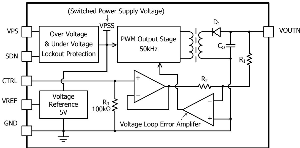
$$VOUTN = -N \times V_{CTRL}, \text{ where } N \text{ is the amplification factor: } N = R_1/R_2.$$
