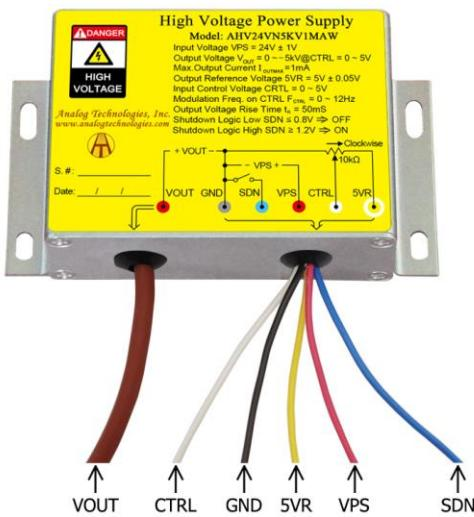
Figure 2. The Connecting Lead Wires of AHV24VN5KV1MAW
