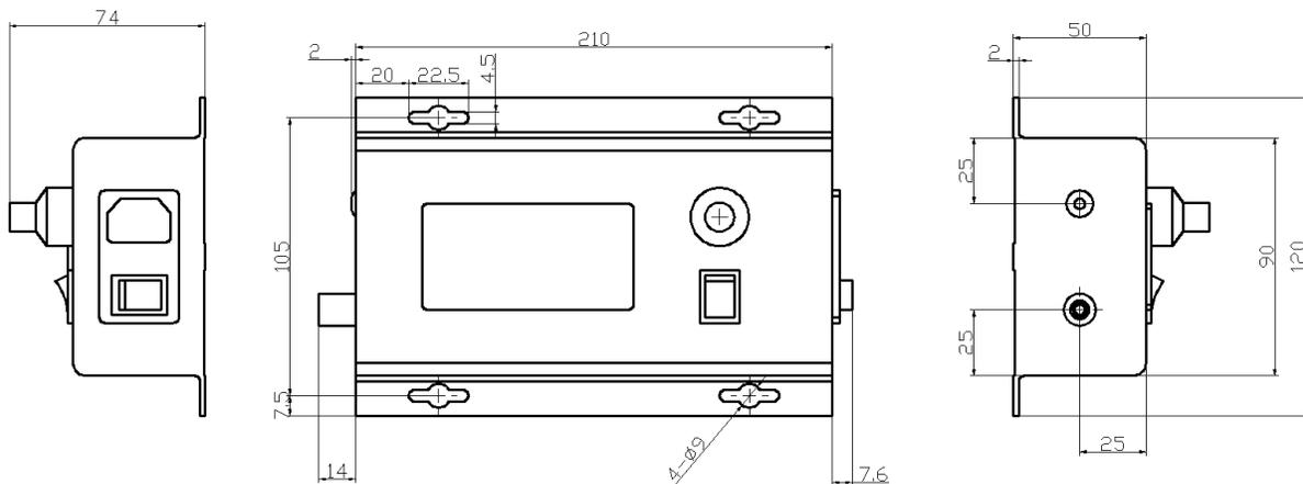
Figure 9. Dimensions for AHVAC20KVR5MABT
