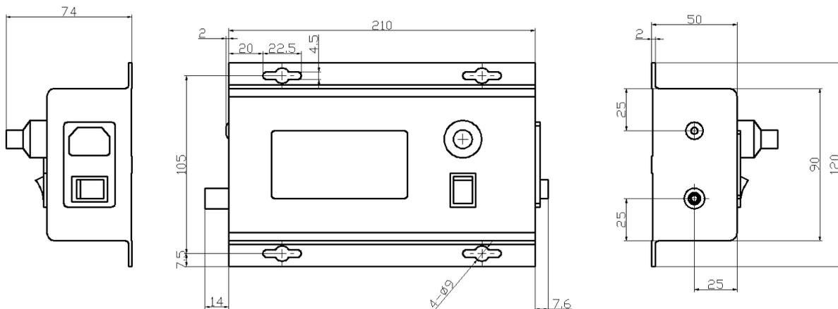
Figure 9. Dimensions for AHVACN5KV5MABT
