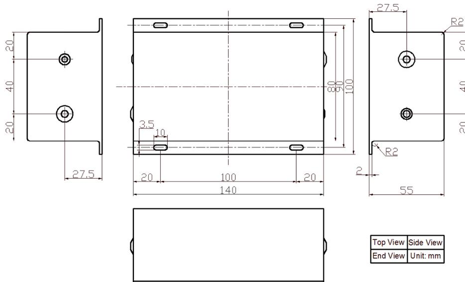
Figure 12. Dimensions for ALSHV24V6600V10MAW
