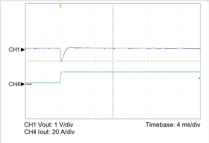
Figure 6 — 10% to 100% load transient response,  $V_{IN} = 270\text{ V}$ , nominal trim,  $C_{OUT\_EXT} = 220\ \mu\text{F}$
