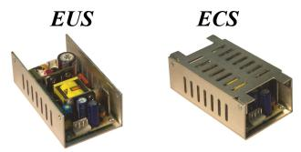
Our Standard power supplies, the DY060 Series, can be installed into a fully-enclosed chassis or in a 'U' shape chassis as an option. These options offer two mounting planes. The fully enclosed option helps to reduce radiated noise.
