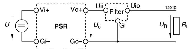
Fig. 2 Reduction of voltage interference by FP filters
