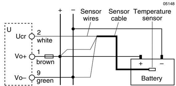
Fig. 3: Connection to the U unit.
