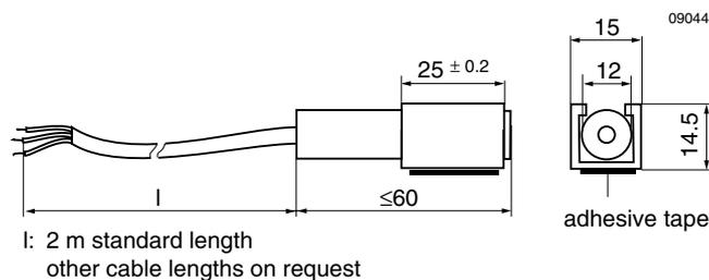
Fig. 4: T and U temperature sensor with mounting fixture.
