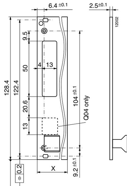
Fig. 1 Front panel for Q case size
