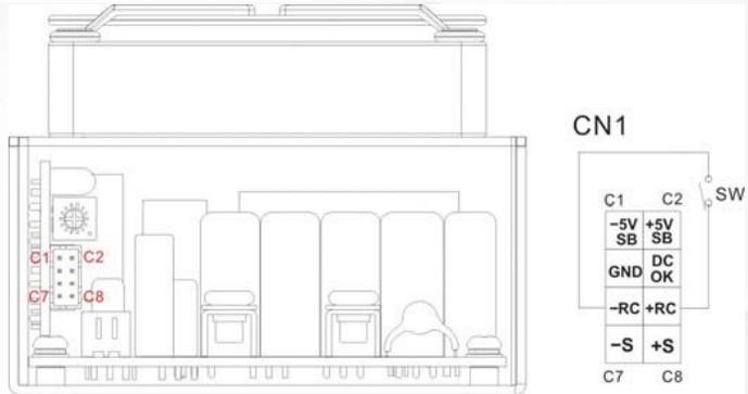
3. +S and -S Sense Shorter wiring to each unit is recommended, as well as twisting +S and -S in pairs, as shown below
