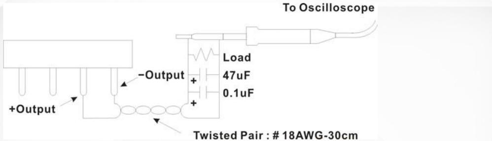
A 30cm twisted pair of no.18 AWG copper wire is connected to a 47uF and 0.1uF capacitor of proper polarity and voltage rating. The oscilloscope probe ground lead should connect right to the ground ring of the probe and be as short as possible. The oscilloscope bandwidth should be at 20MHz and connected to AC ground.
