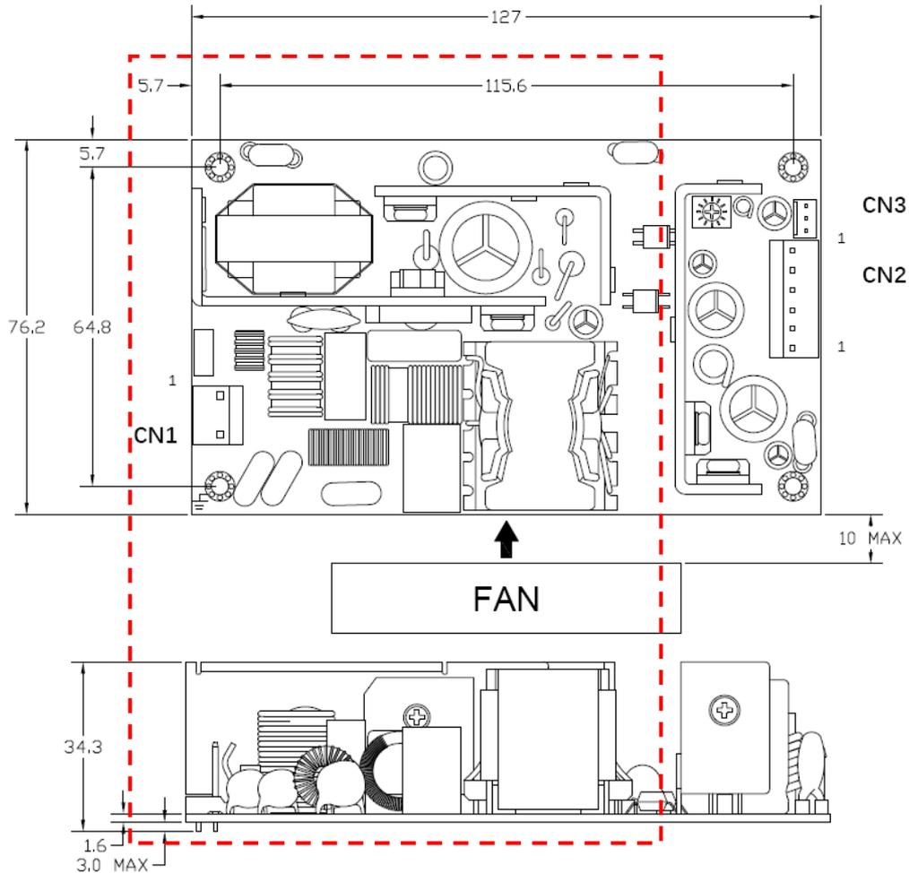
Note:1. The installation shall be kept in an isolation distance min. 2.9mm between the unit and the system chassis. There exist hazardous voltage in dotted area, keep insulating to avoid hazardous electric shock.
