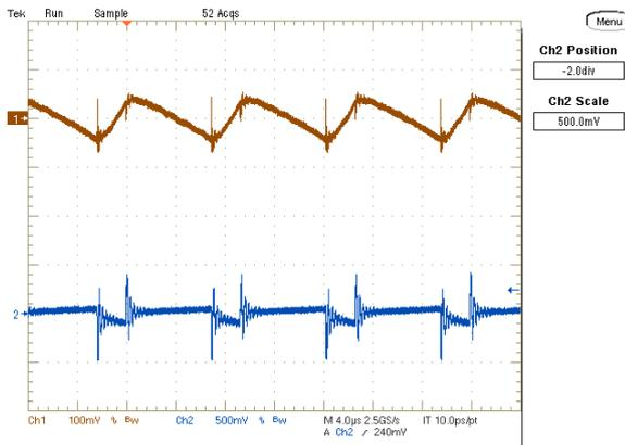
Turn On Delay (Vin = 48V, Iout = 10A,)
