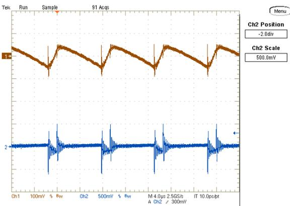
Turn On Delay (Vin = 75V, Iout = 10A,)
