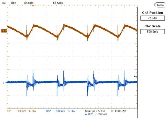
Turn On Delay (Vin = 60V, Iout = 10A,)
