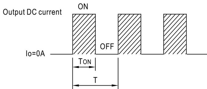
$$\text{Duty cycle(\%)} = \frac{T_{ON}}{T} \times 100\%$$
