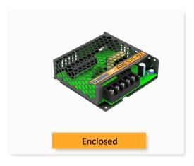
The new AMES75-NZ is a brand-new AC/DC converter that offers much greater cost effectiveness due to material normalization and production automation also leading to improved reliability and performance. Offering a commercial input voltage range of 90-264VAC and an output voltage range from 5-48V, this series will offer many benefits to your new system design.
