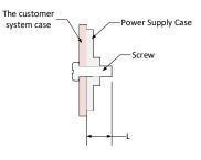
Note: Unit: mm(inch) Wire gauge: 22-12AWG Screw terminal tightening torque: M3.5, 0.8N-m Mounting screw tightening torque: M4, 0.9N-m General tolerance: ±1.0(±0.04)
