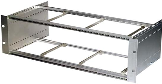
Complete 19" rack with side walls, transversal rails, and mounting flanges. 6 guiding rails are included for set up of a system. The rails shall be fixed to the rack by the included screws (12 screws M2.5 x 12 and 12 nuts).
