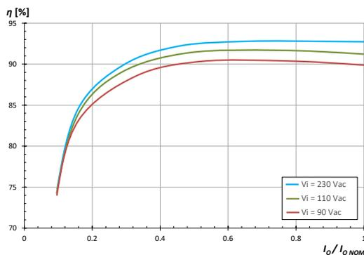
Fig. 2 Efficiency versus  $V_i$  and  $I_o$  (LRP2320 / LRP2540 / LRP2660, both outputs connected in series)
