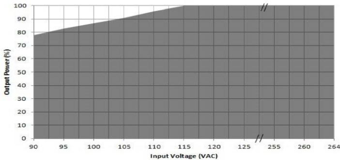
De-rate linearly from 100% at 110 VAC to 78% at 90 VAC
