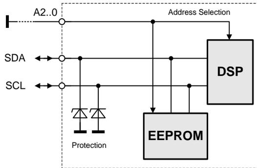
Figure 16. I<sup>2</sup>C Bus to DSP and EEPROM
