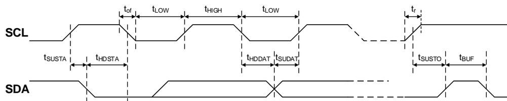
Figure 14. I<sup>2</sup>C / SMBus Timing
