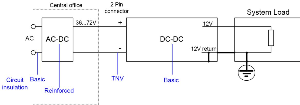
Figure 5. Block diagram with reliable System Earth connection
