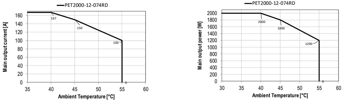
Figure 22. Maximum current and power levels PET2000-12-074RD
