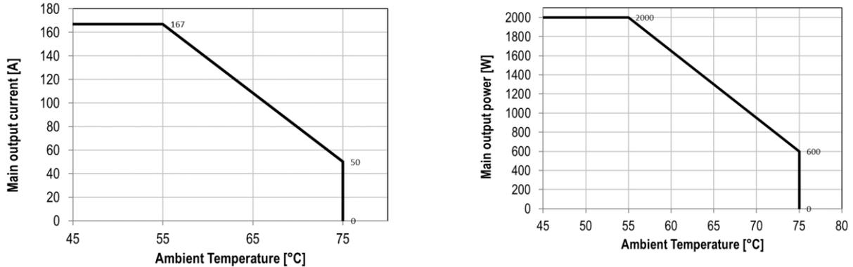
Figure 21. Maximum current and power levels PET2000-12-074ND
