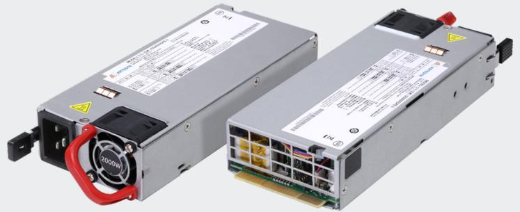
Advanced Energy's Artesyn DS2000SPE is an ultra-high density power supply providing 50W per cubic inch. The 2000 watt DS2000SPE power supply is housed in 1U high rack-mounting enclosures measuring just 3.4 x 7.7 in (86.3 x 196.5 mm). This form factor is significantly shorter than that of similarly rated earlier-generation power supplies — freeing up valuable system space — and is achieved by use of the latest power switching technology and high density component packaging techniques.
