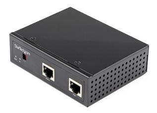
Splits a PoE connection (max 90W) into separate data (RJ45) and DC power (terminal block) that can power any device that uses DC power between 12V-48VDC (1.5A). Power non-PoE devices using network infrastructure, where power is not available.
