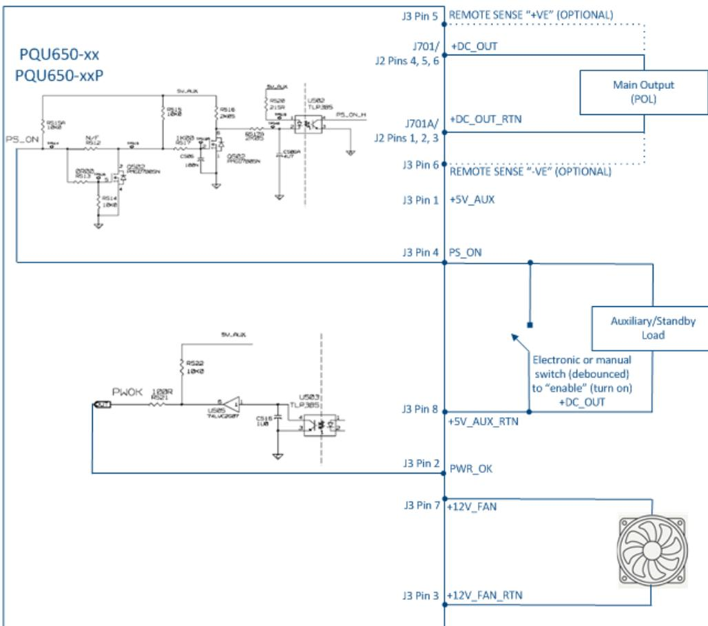
Note: For parallel (current share) operation it is required to connect the sharing power supplies in parallel (+DC out connected together and DC out Return connected together). Since each output has an identical "droop" share characteristic then each output will intrinsically share the total load current. See ACAN-107 for more details. It is recommended that for redundant (critical) applications that external isolation devices (diodes or MOSFETS) are employed; see ACAN-105 for suggested devices.
