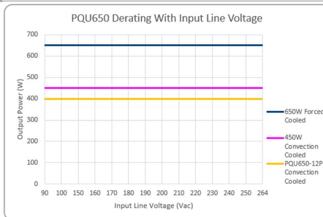
No derating with input line voltage for convection or forced cooling airflows for all variants in the series, except for PQU650-12P that derates to 400W when convection cooled.
