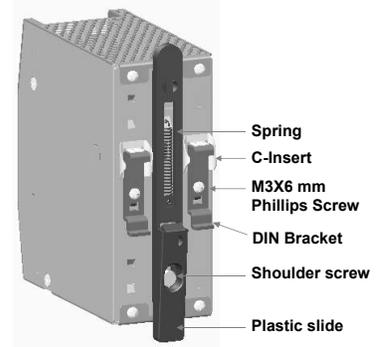
2. Retain and slide back the two DIN brackets to use as a guide for the installation of the panel mount brackets.
