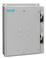
Duplex starter w/o alternator, Size 1, Three phase full voltage, Solid-state overload relay, OLR amp range 10-40A, 110V 50Hz / 120V 60Hz coil, Combination type, Two 30A circuit breakers, Enclosure NEMA type 1, Indoor general purpose use
