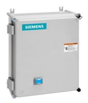
Non-reversing motor starter, Size 1, Single phase full voltage, Solid-state overload relay, OLR amp range 3-12A, 208VAC 60Hz coil, Non-combination type, Enclosure type 4X fiberglass, Water/dust tight noncorrosive, Standard width enclosure
