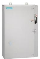
Non-reversing motor starter Size 1 Three phase full voltage Solid-state overload relay OLRelay amp range 10-40a 240VAC 50HZ / 277VAC 60HZ coil Combination type 60Amp non-fused disconnect Encl NEMA type 4X 316 S-steel Water/dust tight non-corrosive Extra-wide enclosure
