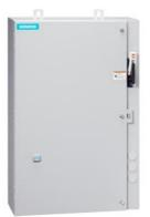
Non-reversing motor starter, Size 1, Three phase full voltage, Solid-state overload relay, OLR amp range 10-40A, Combination type, 60A fusible disconnect, 60A/250V fuse clip, Encl NEMA type 4X 304 S-Steel, Water/dust tight noncorrosive, Extra-wide enclosure
