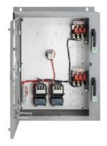
Duplex starter with alternator Size 1 3/4 Three phase full voltage Solid-state overload relay OLR amp range 10-40A 110VAC 50Hz / 120VAC 60Hz Coil Combination type Two 60A disconnect switches Enclosure NEMA type 1 Indoor general purpose use
