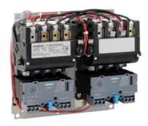
2-speed 3-phase motor starter Size 0 Two separate windings Constant or variable torque Solid-state overload relays Low SPD OLR range 0.75-3.4A High SPD OLR range 3-12A 110-120/220-240VAC 60HZ coil Enclosure NEMA type (open) No enclosure
