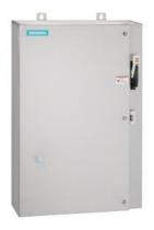
Non-reversing motor starter Size 0 Three phase full voltage Solid-state overload relay OLRelay amp range 5.5-22A 240VAC 50HZ / 277VAC 60HZ coil Combination type 30Amp non-fusible disconnect Encl NEMA type 4X 316 S-steel Water/dust tight non-corrosive Extra-wide enclosure
