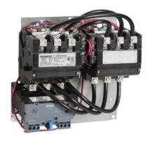
Reversing motor starter Size 3 1/2 Three phase full voltage Solid-state overload relay OLRelay amp range 50-200A 110VAC 50HZ / 120VAC 60HZ coil Noncombination type Enclosure type (open)
