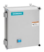
Non-reversing motor starter, Size 1, Three phase full voltage, Solid-state overload relay, OLR amp range 0.25-1A, 110V 50Hz / 120V 60Hz coil, Non-combination type, Enclosure type 4X fiberglass, Water/dust tight noncorrosive, Standard width enclosure
