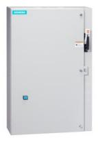
Non-reversing motor starter Size 4 Three phase full voltage Solid-state overload relay OLRelay amp range 50-200A 220-240/440-480VAC 60HZ coil Combination type 150A circuit breaker Enclosure NEMA type 1 Indoor general purpose use Standard width enclosure
