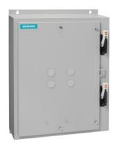
Duplex starter w/o alternator Size 4 Three phase full voltage Solid-state overload relay OLR amp range 50-200A 208VAC 60Hz Coil Combination type Two 200A disconnect switches Encl NEMA type 4 painted steel Water/dust tight weather proof
