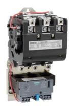
Non-reversing motor starter Size 3 Three phase full voltage Solid-state overload relay OLRelay amp range 25-100A 24VAC 50-60HZ coil Combination type No enclosure
