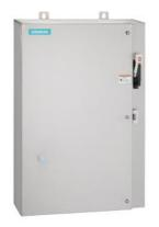
Non-reversing motor starter, Size 3, Three phase full voltage, Solid-state overload relay, OLR amp range 25-100A, 24VAC 50-60Hz coil, Combination type, 100A fusible disconnect, 100A/600V fuse clip, Encl NEMA type 4X 304 S-Steel, Water/dust tight noncorrosive, Extra-wide enclosure
