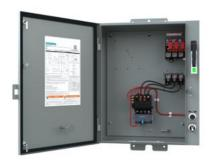
Pump control panel, Size 1, Three phase full voltage, Solid-state overload relay, OLR amp range 5.5-22A, 110V 50Hz / 120V 60Hz coil, Standard type contactor, 60A fusible disconnect, 60A/600V fuse clip, HOA Sel Sw. <(>&<)> Start P.B., Enclosure NEMA type 3/3R, Weather proof outdoor use
