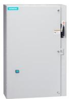
Non-reversing motor starter, Size 3, Three phase full voltage, Solid-state overload relay, OLR amp range 25-100A, 208VAC 60Hz coil, Combination type, 200A fusible disconnect, 200A/250V fuse clip, Enclosure NEMA type 1, Indoor general purpose use, Extra-wide enclosure
