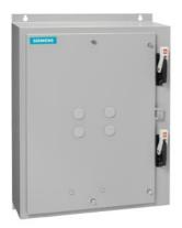
Duplex starter w/o alternator Size 0 Three phase full voltage Solid-state overload relay OLR amp range 0.75-3.4A 208VAC 60Hz Coil Combination type Two 30A disconnect switches Enclosure NEMA type 4/12 Water/dust tight weather proof
