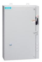
Reversing motor starter, Size 1 3/4, Three phase full voltage, Solid-state overload relay, OLR amp range 10-40A, 110V 50Hz / 120V 60Hz coil, Combination type, 60A disconnect switch, Encl NEMA type 4X 304 S-Steel, Water/dust tight noncorrosive
