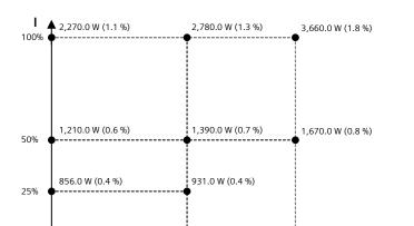
The percentage values show the losses in relation to the rated apparent power of the converter.
