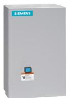
Non-reversing motor starter, Size 2 1/2, Three phase full voltage, Amb. compensate bimetal OLR, Contactor amp rating 60A, 24VAC 50-60Hz coil, Non-combination type, Enclosure type 1, Indoor general purpose use
