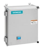
Non-reversing motor starter, Size 1, Three phase full voltage, Solid-state overload relay, OLR amp range 10-40A, 24VDC coil, Non-combination type, Enclosure type 4X fiberglass, Water/dust tight noncorrosive, Standard width enclosure
