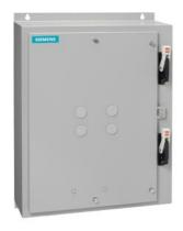
Duplex starter w/ alternator, Size 1, Three phase full voltage, Solid-state overload relay, OLR amp range 5.5-22A, 110V 50Hz / 120V 60Hz coil, Combination type, Two 25A circuit breakers, Enc NEMA type 4 painted steel, Water/dust tight for outdoors
