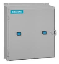
Duplex starter w/o alternator, Size 3 1/2, Three phase full voltage, Solid-state overload relay, OLR amp range 50-200A, 110V 50Hz / 120V 60Hz coil, Noncombination type, Encl NEMA type 4X 304 S-Steel, Water/dust tight noncorrosive
